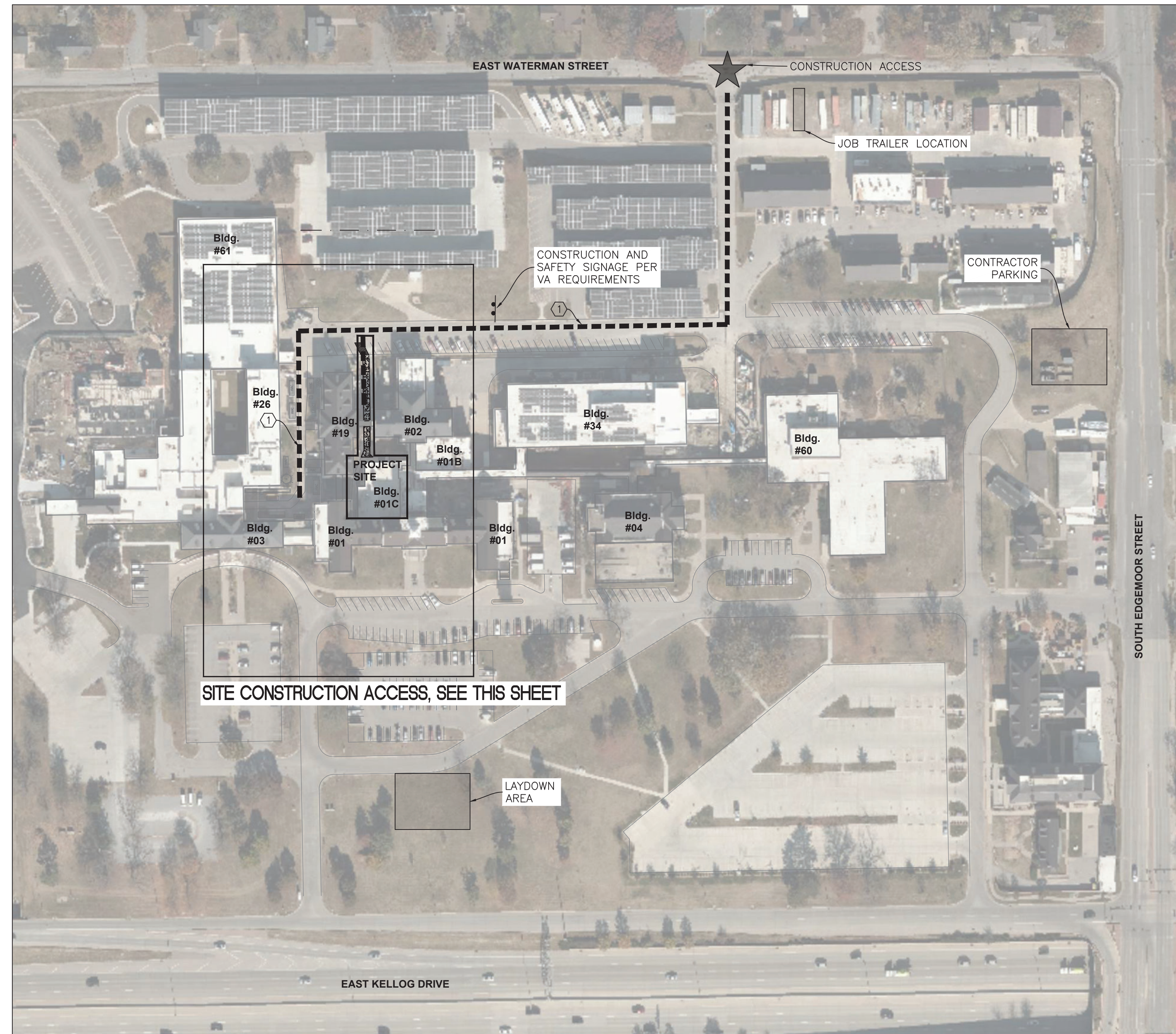
CAMPUS CONSTRUCTION ACCESS (SCALE 1"=100')
