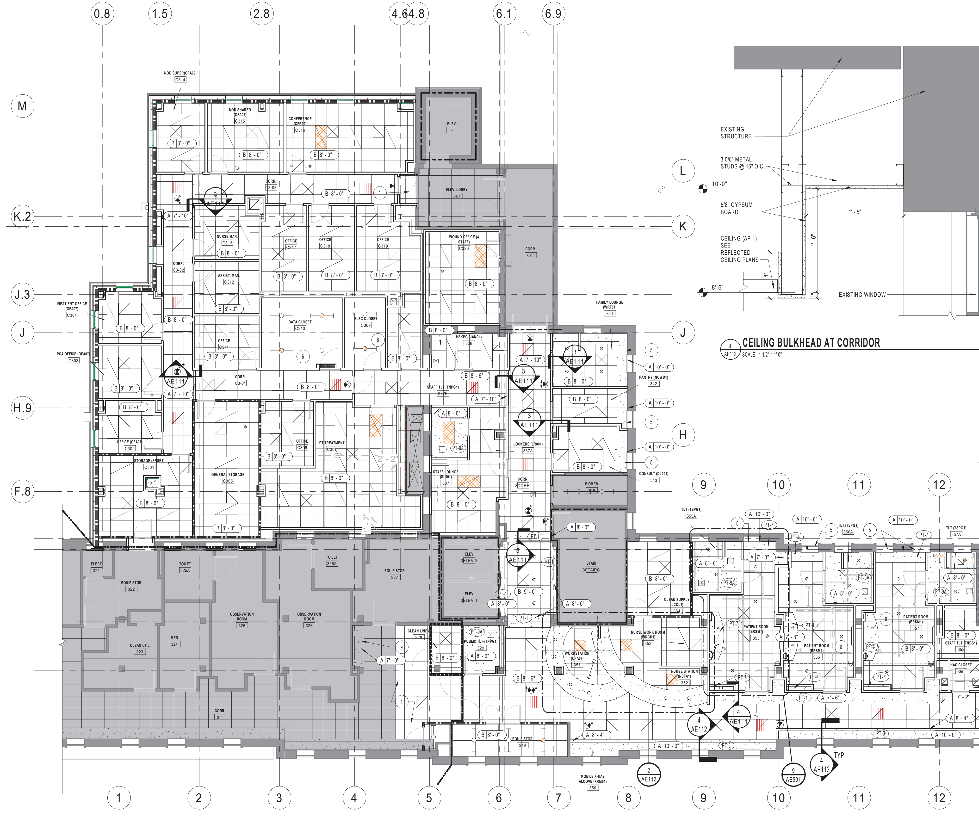
3 ENLARGED CEILING PLAN - ABOVE NURSE STATION 2 AE112 SCALE: 1/4" = 1'-0"
