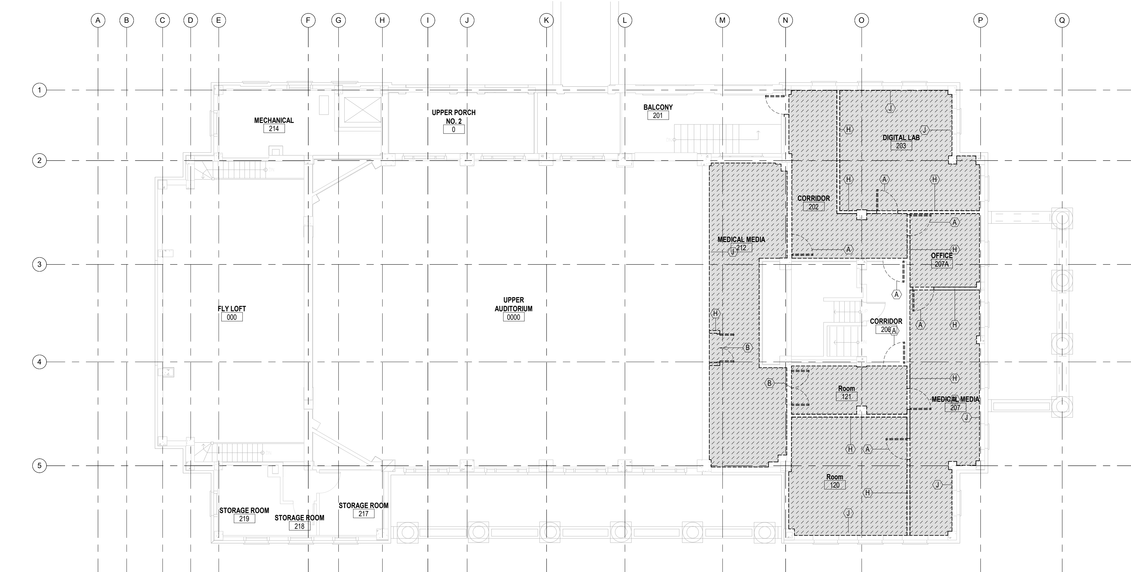
3 SECOND FLOOR DEMOLITION 1/8" = 1'-0"
