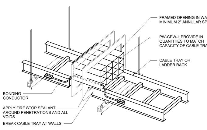
NOTES: 1. REFER TO SPECIFICATION SECTION 17080 THROUGH PENETRATION FIRESTOPPING FOR ADDITIONAL INFORMATION. 2. REFER TO SPECIFICATIONS FOR LADDER RACK AND CABLE TRAY INFORMATION. LADDER TYPE CABLE TRAY IS ONLY SHOWN FOR CLARITY OF ILLUSTRATION. 3. PROVIDE GROUNDING LUGS WITH <u>PW-CPW-1</u> AND BOND TO GROUND PER MANUFACTURERS INSTRUCTIONS.
