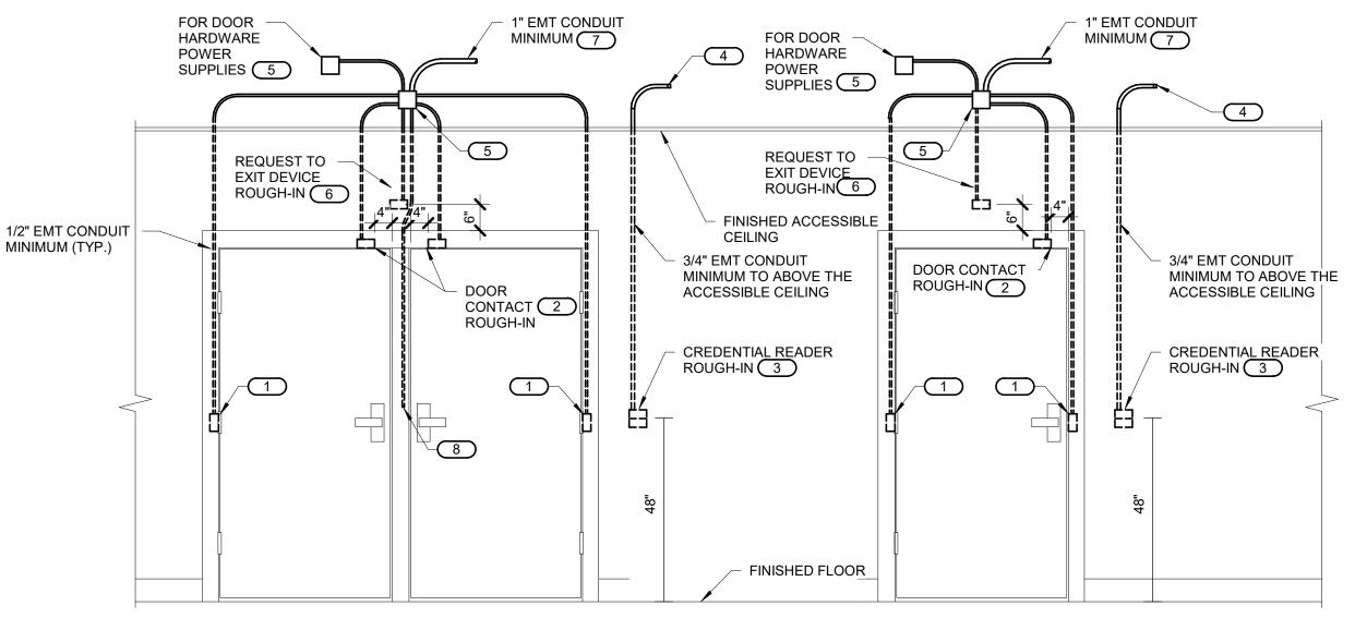
DOOR FRAME ROUGH-IN DIAGRAM (ALL DOUBLE DOORS WITH OR WITHOUT MULLION) DOOR FRAME ROUGH-IN DIAGRAM (ALL SINGLE DOORS)
