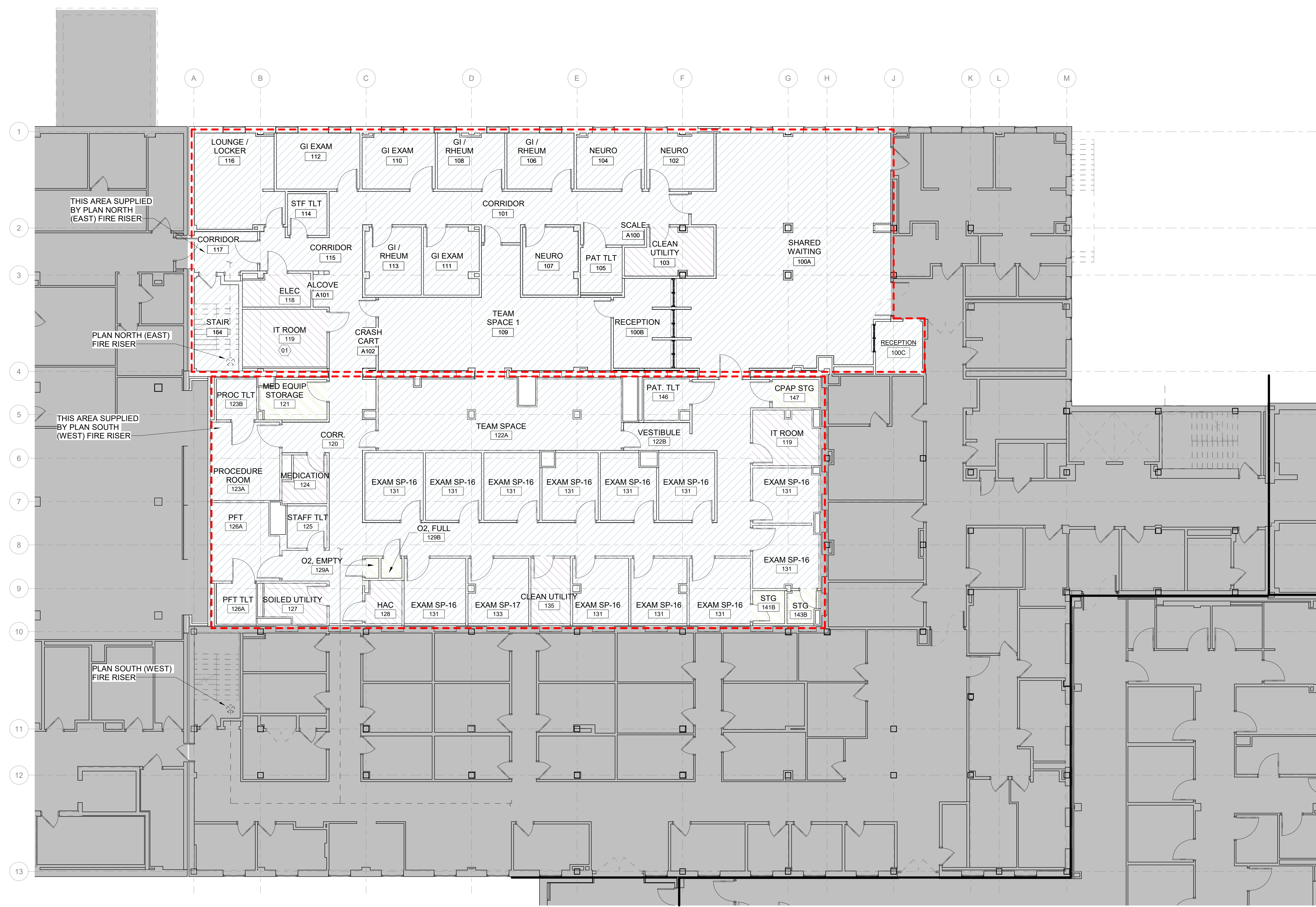
FIRE SUPPRESSION HAZARD CLASSIFICATION PLAN - FIRST FLOOR 1 1/8" = 1'-0"
