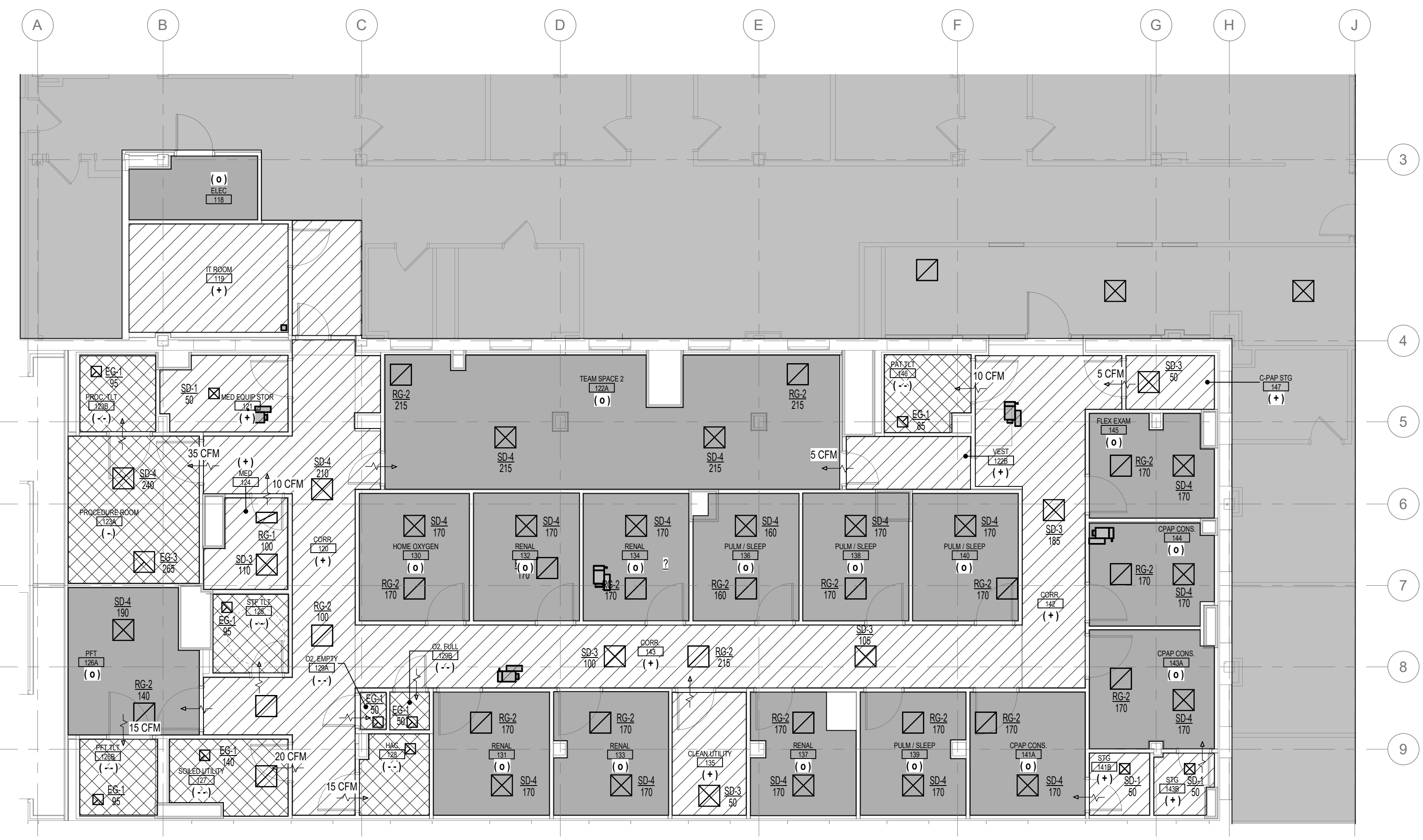
2 FIRST FLOOR HVAC ZONING PLAN - PHASE ONE 1/8" = 1'-0"
